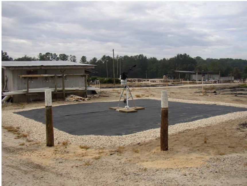
Davis Vantage Pro2 Plus weather station with a hardwired connection to a Davis data-logging console housed in an adjacent building.
